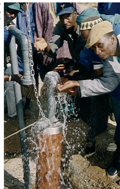
Pumping test at a borehole in a village in Mali
